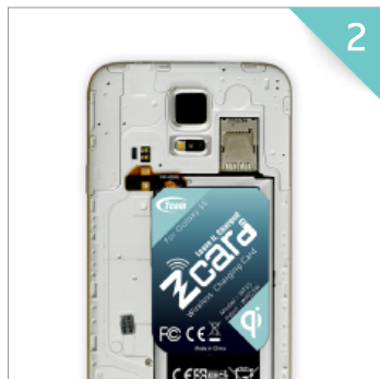
2 Remove the double sided tape from the Zcard and attach the Zcard to the back of the battery firmly, ensuring the contact points are properly connected.
