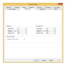
When the **Manual Input** tab is selected there is no encoder feedback therefore multiple A-scans are not recorded. Use this mode for manual 'free-hand' scanning with imaging when a record (snapshot) of the currently displayed data may be required. When the scan is terminated, only the data currently displayed is saved.
