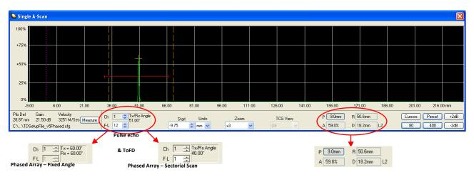
The A-Scan display window shows the digitised ultrasonic signal received by the transducer.
