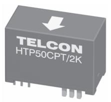
The HTP50CPT/2k is a closed loop Hall Effect Current Transformer suitable for measuring currents up to 50A. The product provides an output current into an external load resistance which is galvanically isolated from the primary conductor. All contacts, including the primary, are designed for PCB mounting.
