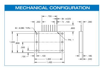
The UDOS007 drawing shows the hermetic package, mounting flange and 8 external connections. All dimensions given are in inches and tolerances are ±0.005. The package walls are 0.040 inch thick and the cover is 0.010 inch thick.
