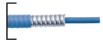
Designed for both inside and outside environments where the application requires the ultimate in cut and crush resistance (500 lbs/in). This cable is covered with a stainless steel interlocked armor; an additional polyolefin jacket is standard. Temperature range -54° C to +135° C.
