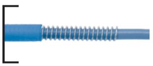
For applications requiring a slightly greater amount of compression resistance (300 lbs/in), but where weight and flexibility are also critical. The cable is covered with a flexible wound helix of passivated stainless steel wire and a cross-linked polyolefin jacket. Temperature: -54° C thru +135° C.
