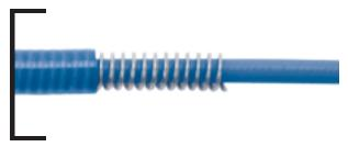
For applications similar to the above, where weight, flexibility, and moderate compression resistance (300 lbs/in) are important, but where abrasion resistance is also critical. The cable is covered with a flexible wound helix of passivated stainless steel wire and an extruded polyurethane jacket. Temperature: -54° C thru +100° C.
