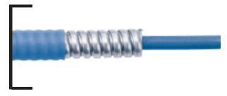
Designed for both inside and outside environments where flexibility and weight are not as critical, but where the application requires the ultimate in cut and crush resistance (500 lbs/in). The cable is covered with a stainless steel interlocked armor; an additional cross-linked polyolefin jacket is standard on lengths up to fifty feet. Temperature: -54° C thru +135° C.
