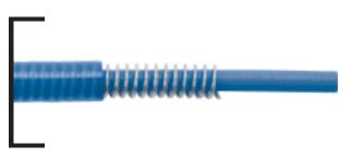
Designed for applications where weight, flexibility, and abrasion resistance are critical and moderate compression resistance is required (300 lbs/in). The cable is covered with a flexible wound helix of passivated stainless steel wire and an extruded polyurethane jacket. Temperature range -54° C to +100° C.
