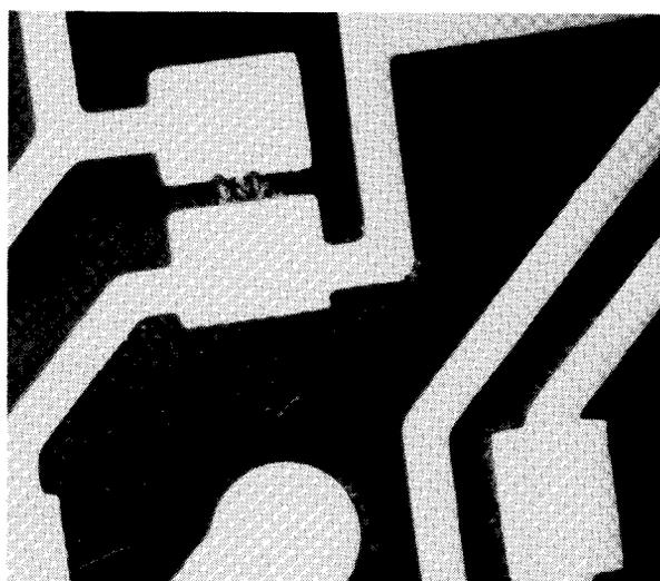
Fig. 8. Silver electromigration on porcelainized PC board. 4.8 x . Note dendritic bridging of 0.38-mm (0.015in) spacing, and orientation of dendrites on circular pad towards anodic conductor.
