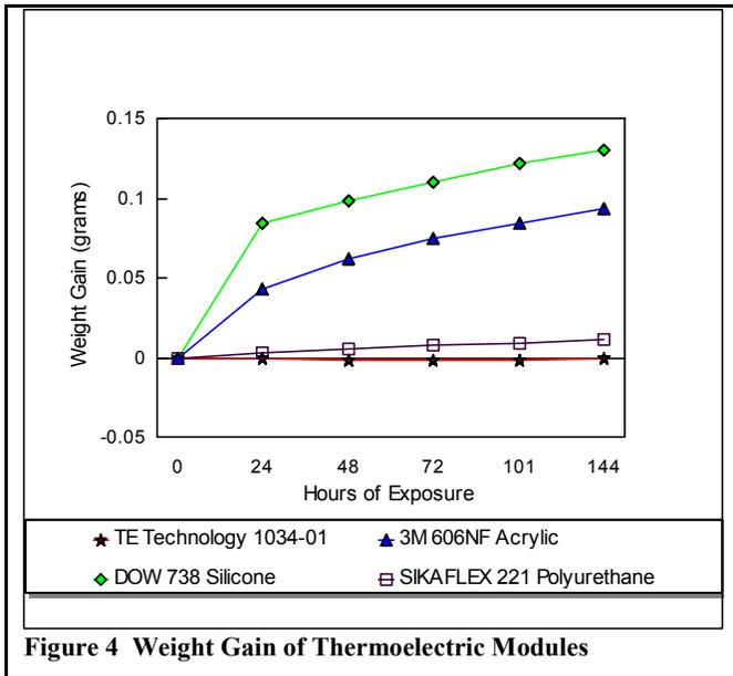
**Figure 4 Weight Gain of Thermolectric Modules**
