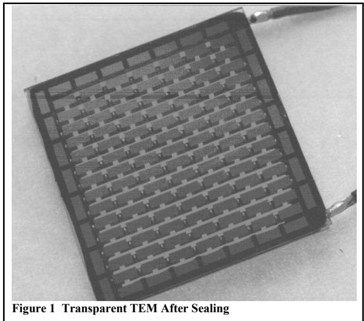
Figure 1 Transparent TEM After Sealing
