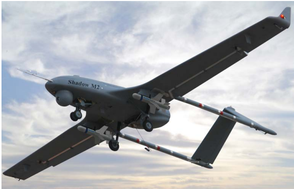
Shadow M2 has a total payload capacity of 130 lb (59 kg) with a full fuel load.
