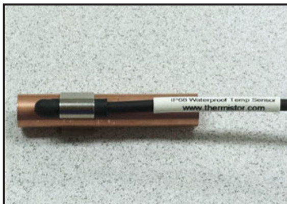
Figure 2. IP68 sensor mounted to 3/8" tube with QTI clip.
