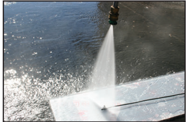
Figure 13. Pressure washing a QTI IP68 sensor at a distance of 25 cm.
