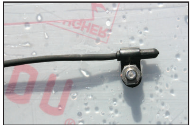
Figure 15. The IP68 sensor after pressure washing at 25 cm.
