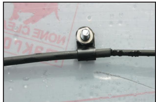
Figure 17. The reinforced sensor after pressure washing at a distance of 10 cm.
