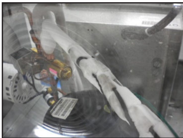
Figure 9. Iced sensors mounted to copper tubing.
