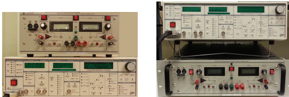
Figure 32: Boosted operation: recommended stack-up
