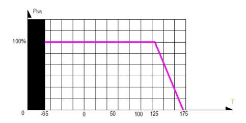
This value is only valid by using a thermal conduction to the heat sink Rth-cs<0.025°K/W.
