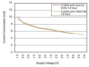
Figure 2. Power Consumption in RX
