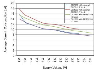
Figure 9. Average Power Consumption in Bluetooth Smart Connection Mode (connection interval 1 s)
