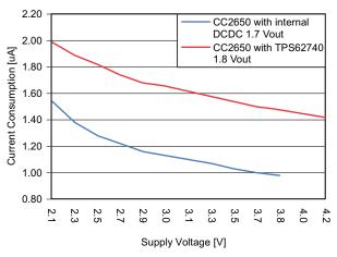
Figure 4. Power Consumption in Standby
