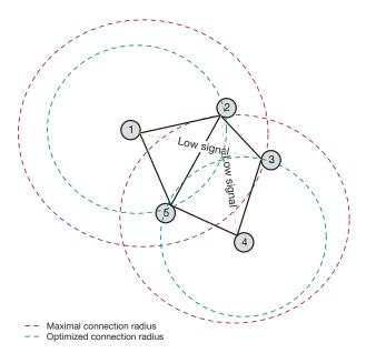
Figure 10: Network's maximal and optimized connection radius
