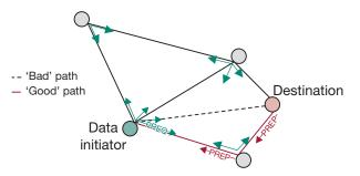
Figure 6: PREQ frames are distributed over the network reaching to the destination. The destination replies using the best path.
