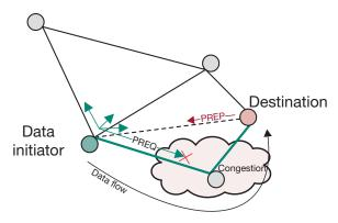
Figure 9: PREQ lost, PREP returns on the nonoptimal path
