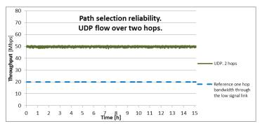
Figure 15: Path selection reliability. Actual result for the data flow over two hops for 15 hours
