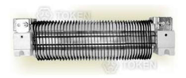
brazed to the oval, spiral edge-wound resistance element. Toothed ceramic insulators isolate the resistance element from the center support. Ceramic end bushings insulate the center support from the mountings. Order individual replacement units or entire grids with various mounting configurations. Contact us with your specific needs.
