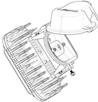
Figure 10: Hang Light Fixture onto Stanchion Mount
