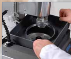
Convenient Cleaning with Removable Slurry Tray
