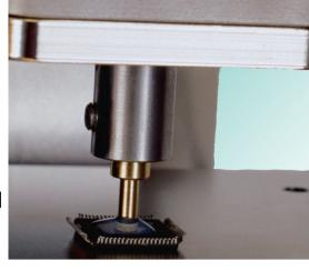
A standard selected area preparation system uses a small rotating tool, oscillating within a predefined amplitude to produce a cavity within the chip before polishing the surface.
