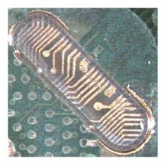
Electronic package after mechanical decapsulation and a 10 second chemical etch reveals the topside circuitry ready for analysis, left. Precisely milled sections of multi-layer PCBs allow for electrical connection of circuitry that would ordinarily be unreachable, right.
