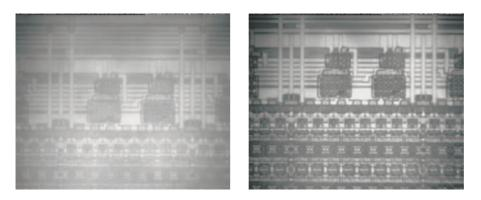
Typical backside image without anti-reflective coat, left. Same area of sample after antireflective coating, right.
