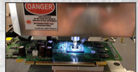
Graphics card mounted and electrically connected to the end-point sensor plate.
