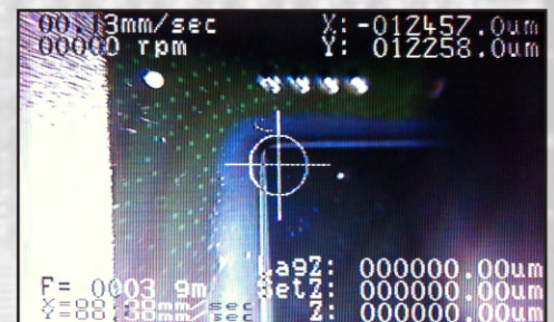
Machine Vision – The on-board monitor is always live, uniquely showing the tool/surface interface overlaid with machine settings. Output to a PC allows video to be saved
