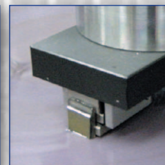
6145.1 Single Die Stub Cross-section holder
