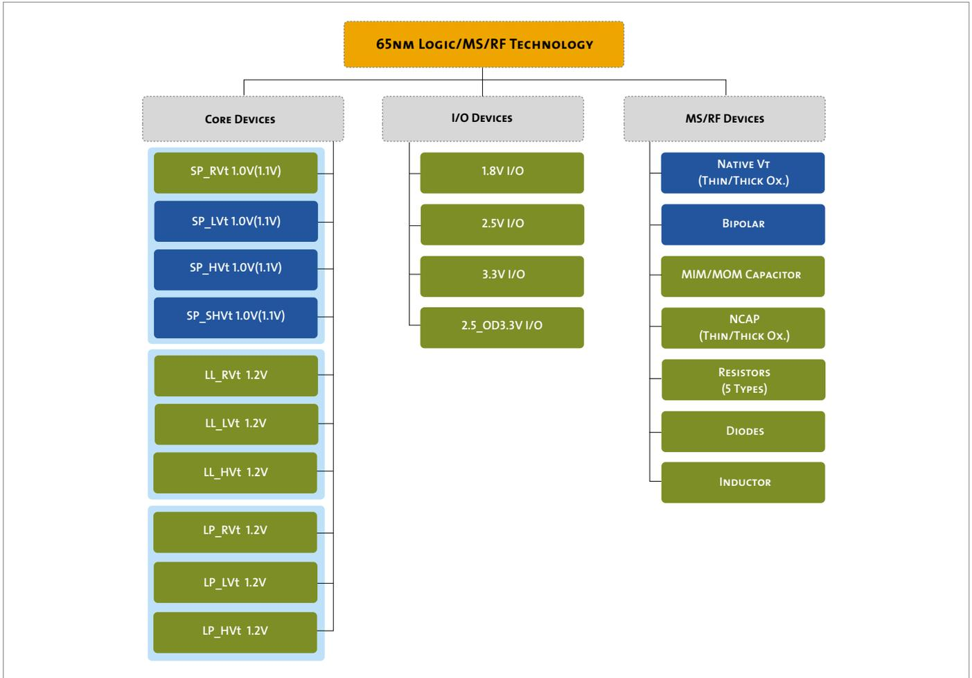
SP: Standard Performance    LL: Low Leakage    LP: Low Power    ■ : RF Model Available (LL and SP)
