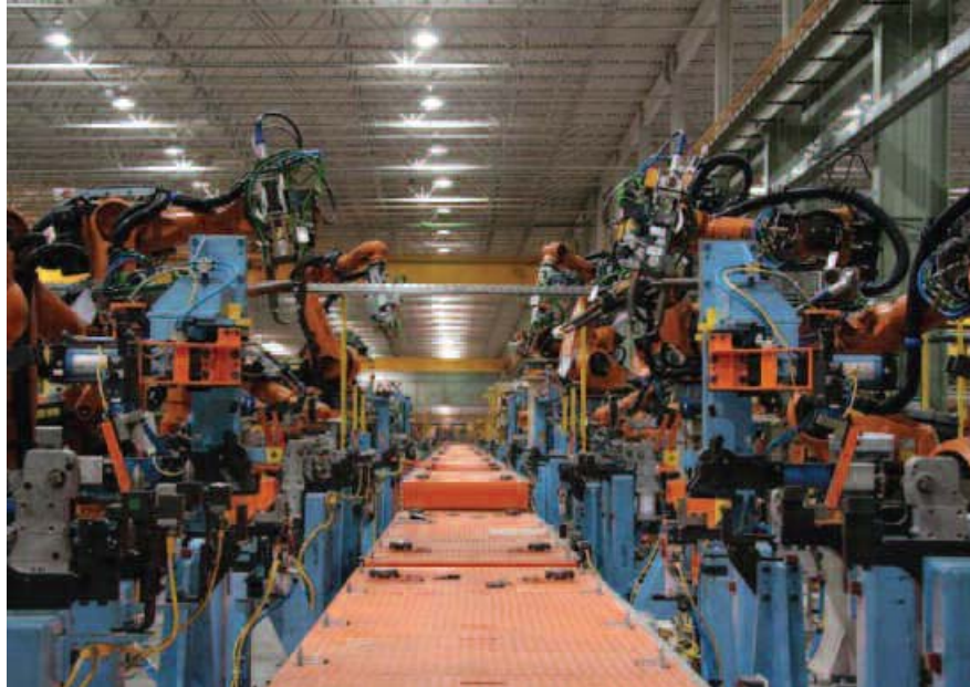
Utilizing robots, adhesives are applied and body panel components are welded inline.
