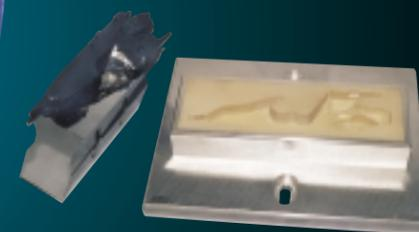
Fig. 10 Contoured milled horn (with part) and poured rigid epoxy nest.
