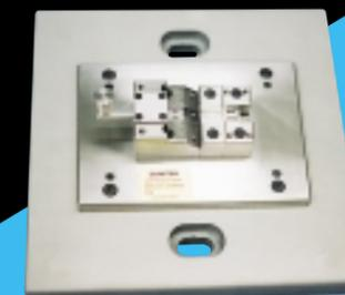
Fig. 11 Machined fixture with horizontal locking/support lever.
