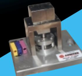
Fig. 14 Fixture with pneumatic eject.
