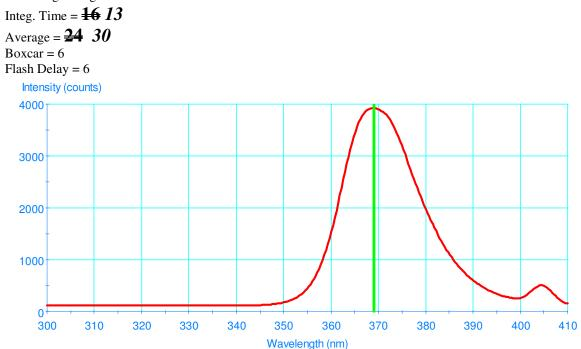
Peak wavelength is about 368 nm. OO reads 369.16 nm with a peak of about 3920 counts. Measured on 4-3-03 by DEN.
