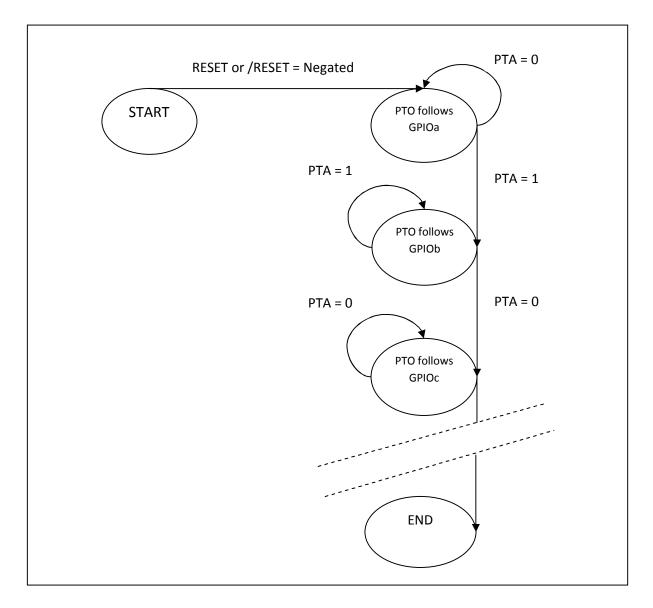
When /RESET is negated, the State Machine advances immediately, or as soon as possible to the first state. At this time the In-Circuit Tester can drive GPIOa and expect the PTO output to follow. The microcontroller remains in this state until the In-Circuit tester drives a logic-high to the PTA input. At this state the In-Circuit Tester can drive GPIOb and expect the PTO output to follow. This sequence continues until all of the GPIO pins are tested.
