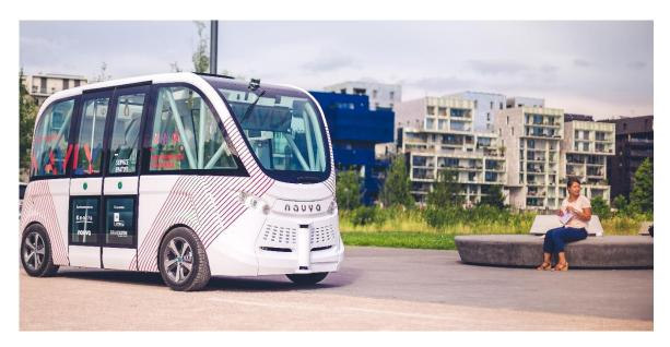
Automated driving and electric powertrains are two key focuses of Valeo's innovation strategy, which is why the Group acquired a stake in Navya in October 2016. Working at the crossroads of vehicle autonomy and electrification, Navya has developed the Navya Arma, a 100% automated, driverless, electric shuttle that can transport up to 15 people.
