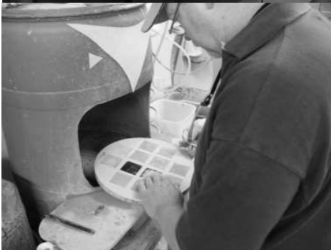
Polishing a very thin, rectangular substrate.
