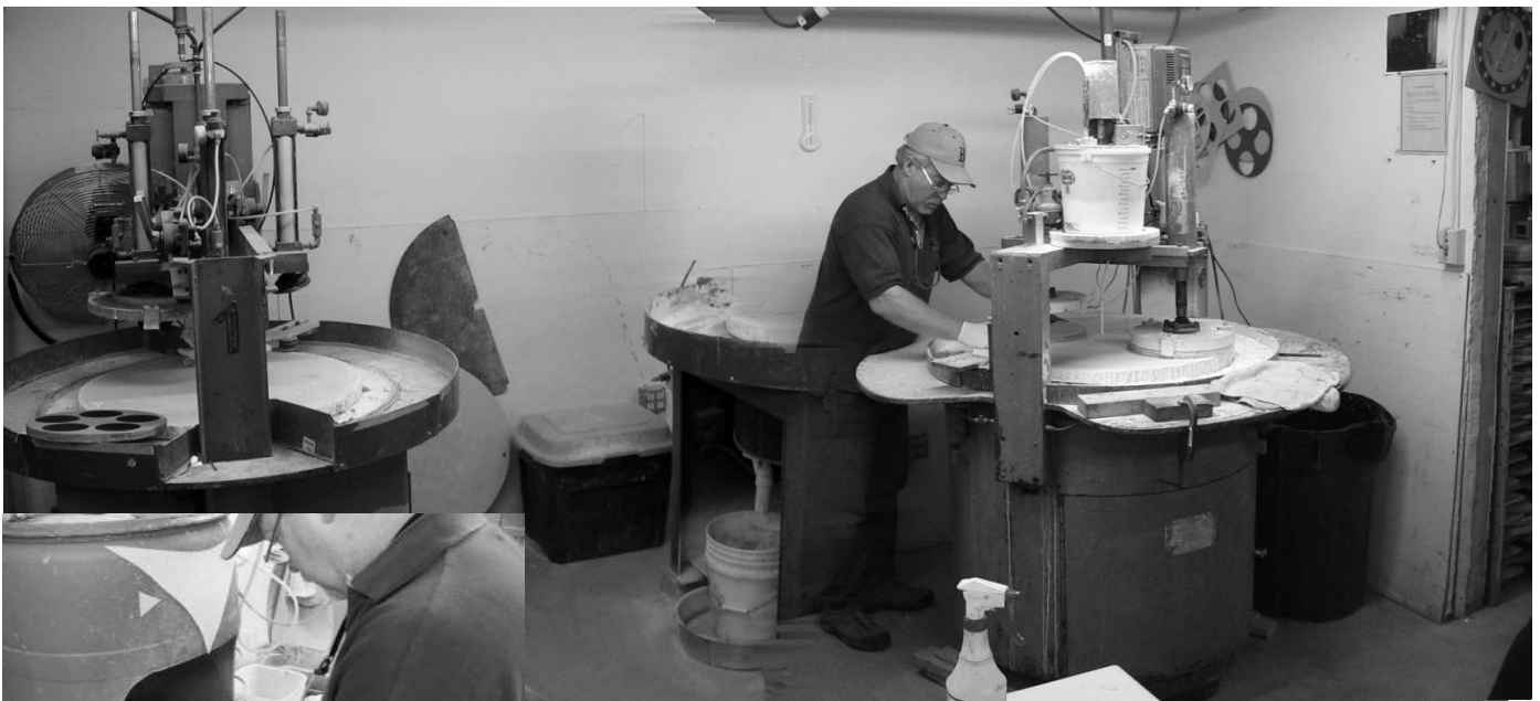
Polishing a very thin, rectangular substrate.
