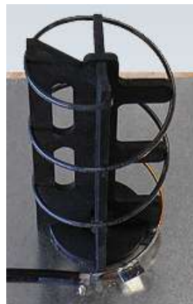
Fig 20 Circularly Polarized Antenna and Electric Field Pattern
