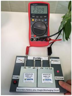
(The picture shows an ultrathin secondary battery from the BatMat project)
