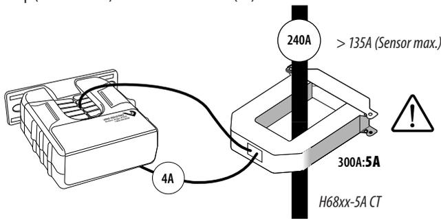
**DANGER:** 5A CTs can present hazardous voltages. Install CTs in accordance with manufacturer's instructions. Terminate the CT secondary before applying current.
