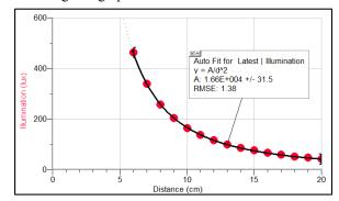
The light intensity follows the expected inverse-square relationship well. Another way to show this relationship is to graph light intensity *vs.* the inverse of the squared distances. The resulting graph should be a direct proportionality. The next graph shows this result.
