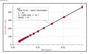
The room was partially darkened during data collection. If there is substantial background light, both graphs would be shifted upward, and the fits would require an additive term.
