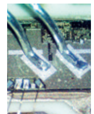
Wire bond (Wedge characteristic)
