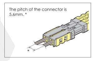
Insert the wire until it reaches the end and use a plier at its open jaw condition.
