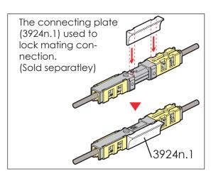
For multi pole connection link the connectors together by sliding them along the easy guide rail.
