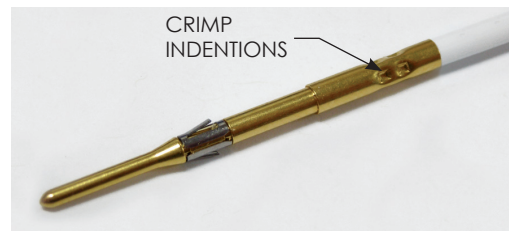
Figure D. Correct location of the crimp divots.
