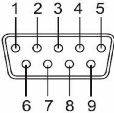
**RS-232 Signal Pin-outs of DB-9 Male (CN2)**
