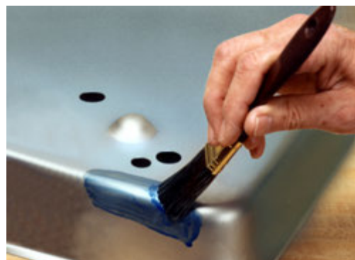
Blue Stop-Off brushed onto surface part
