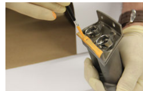
Orange Stop-Off brushed on vane segment
