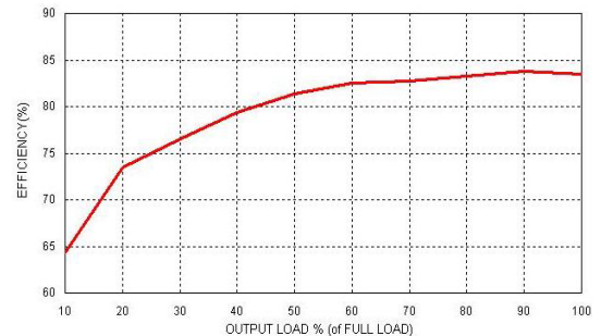
DCNSR-12S05 Efficiency vs Output Load
