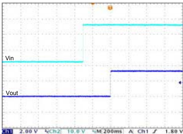
Graph 5: Typical Input Start-Up and Output Rise Characteristic (Nominal Vin and Full Load)
