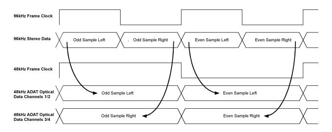
This example shows stereo 96kHz audio data being mapped to four channels of ADAT Optical. The left and right data is shown interleaved, as it might be seen inside a device going to or from DACs or ADCs. Note that this drawing implies that the right channel samples be advanced in time; in fact, the sample-splitting process can only be accomplished by delaying the output (48kHz) samples at least one 96kHz sample period with respect to the input (96kHz) samples.
