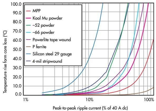
6. When contrasting temperature versus ripple current at 100 kHz, the choice of core material becomes more critical since designs are constrained by core losses at ripple currents as low as 3%.
