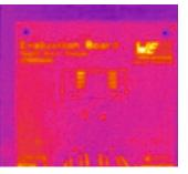
After approximately 5 seconds, one recognises the wires that conduct the power loss in the component. Heating of chip from  $Tu = 20^{\circ}C$  to Tmax at nominal power loss (16.5 W/cm<sup>2</sup>):
