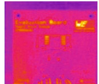
After approximately 5 seconds, one recognises the wires that conduct the power loss in the component. Heating of chip from  $T_u = 20^\circ\text{C}$  to  $T_{max}$  at nominal power loss ( $16.5\text{ W/cm}^2$ ):
