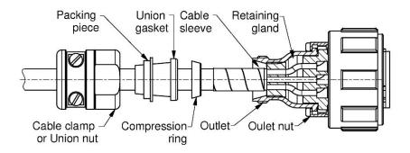
Remove tape from metal braid and fan out 90º to cable. Position compression ring on end of outer sheath, trapping braid between
