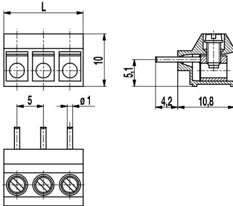
The 951-LH series PCB screw connector with a pitch of 5 mm is particularly suited for potting printed circuits. For such potting applications, the solder pin is sealed at the housing opening against seeping casting resin. This PCB screw connector with a pitch of 5 mm is available in 2- to 12-pole design and can be mounted side-by-side without pole loss.
