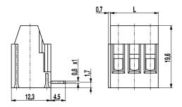
The PCB connector 150-A-121 is the horizontal version of 150-A-111 with a pitch of 5 mm and is available with 2 or 3 poles.
