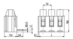
The PCB connector 152-A-221 is the horizontal version of 152-A-211 with a pitch of 7,5 mm is available with 2 or 3 poles.
