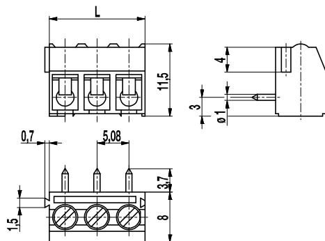
The PCB connector 941-T is the horizontal version of 940-T with a pitch of 5,08 mm and available in 2 and 3 poles. It can be mounted side-by-side without pole loss.
