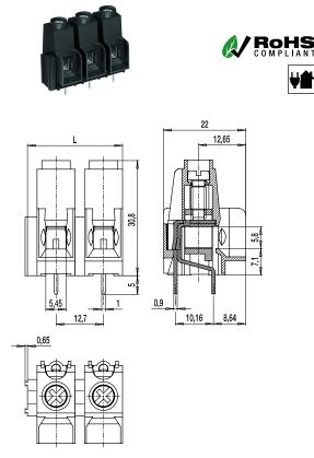
Series 159-A is particularly designed for high voltages and strong currents. A terminal space for solid wires of up to 16 mm<sup>2</sup> or for flexible wires of up to 10 mm<sup>2</sup> is characteristic for this series. Two solder pins per pole ensure safe connection to the PCB.
