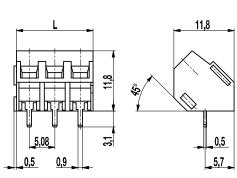
The PCB connector 141-C-111 is the inclined version with lift system with a pitch of 5,08 mm and available in 2 and 3 pole design.
