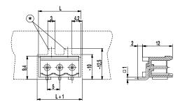
(\*) Please plan for two gaps in the measures of 3 x 2.5 mm in the cut-out of the control panel for the snap-in device of the counterpart
