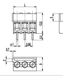
The PCB connector 960-T with a pitch of 5,08 mm is available in 2 and 3 poles and can be mounted side-by-side without pole loss.
